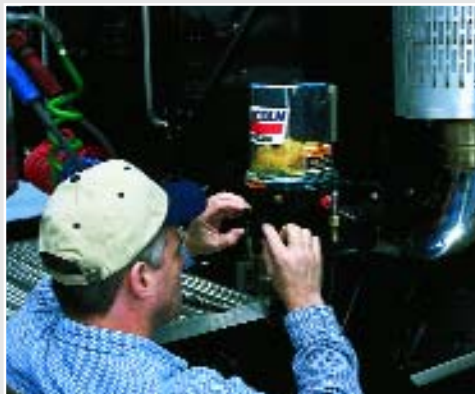
Lincoln's Quicklub 203 Electric Pump comes standard with an integrated timer.
